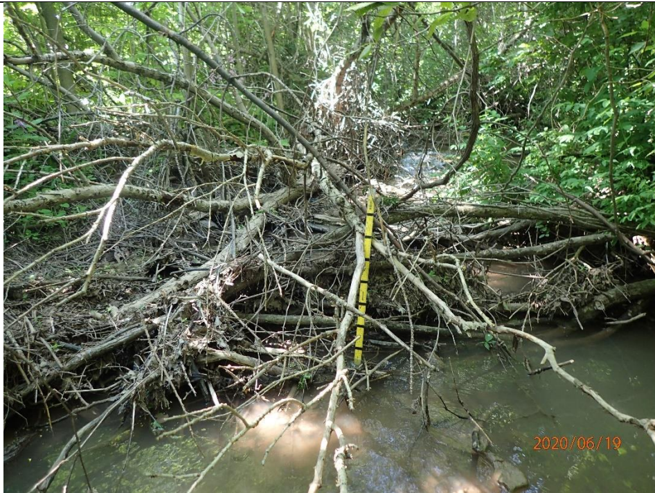
There was a high density of woody debris present in the channel and cut bank. There were approximately 5 woody debris jams per 50 m of the reach.
