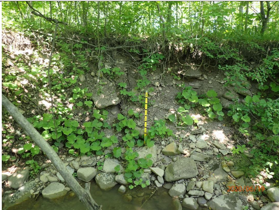
Valley wall contact was common through the upstream sections of the reach. Bank materials consisted of silt, sand, gravel, and cobble.
