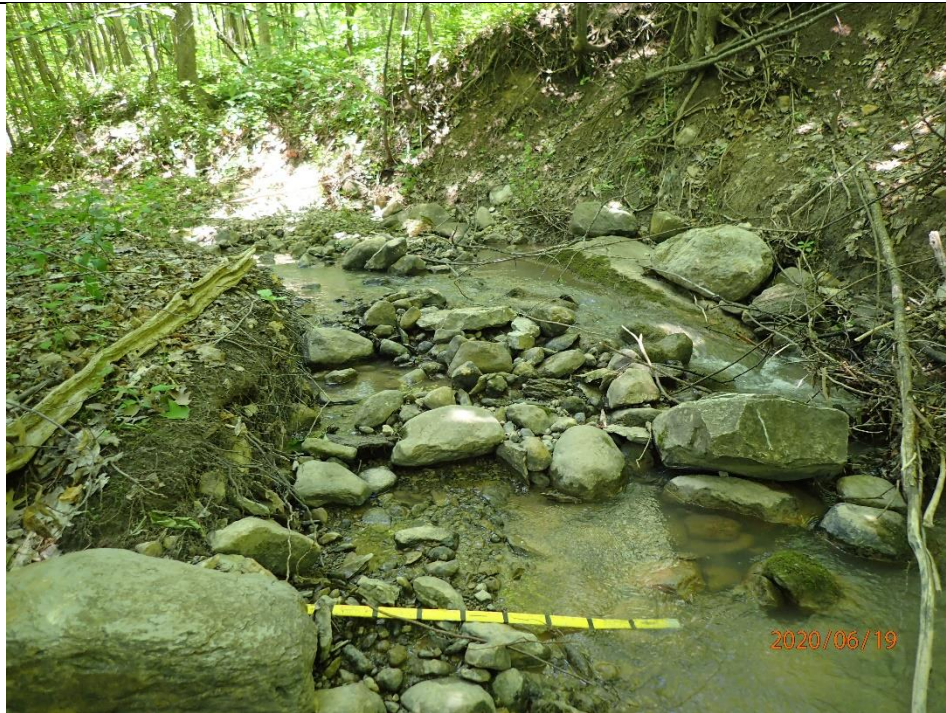
Bar forms were poorly formed or reworked, and the thalweg was out of phase with meander form indicating planimetric form adjustment processes.
