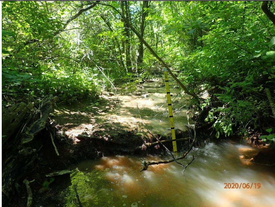
A rooted knickpoint was observed with apparent head-cutting due to knickpoint migration upstream.
