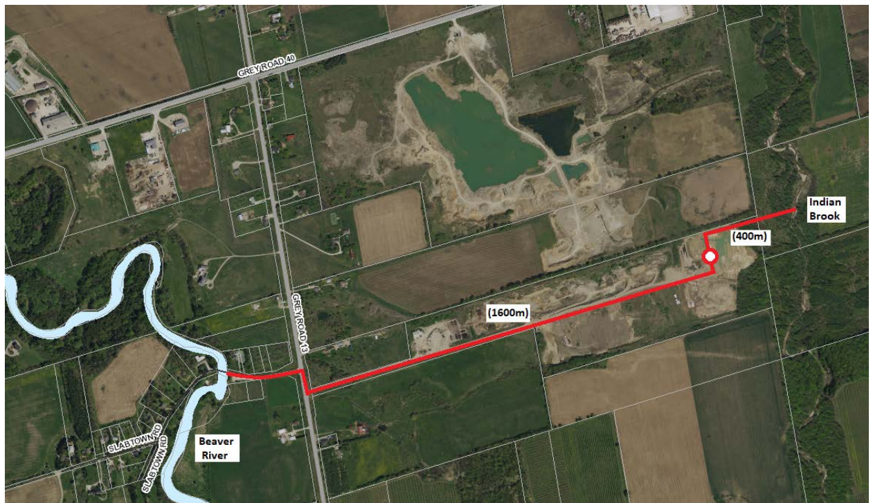
Figure 2 – Effluent Forcemains to Surface Waters
