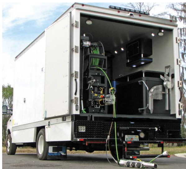
Figure 2: Typical Sewer Inspection Vehicle
