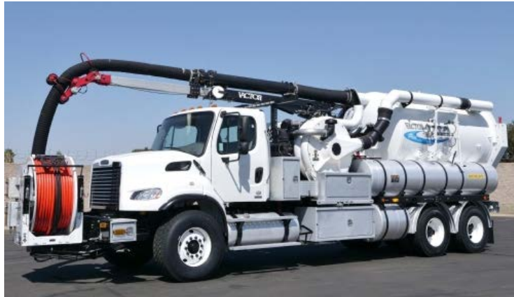
Figure 1: Sewer Jetting & Vacuum Truck
